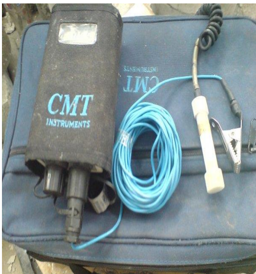
Gambar 3. Alat ukur uji half cell potential
