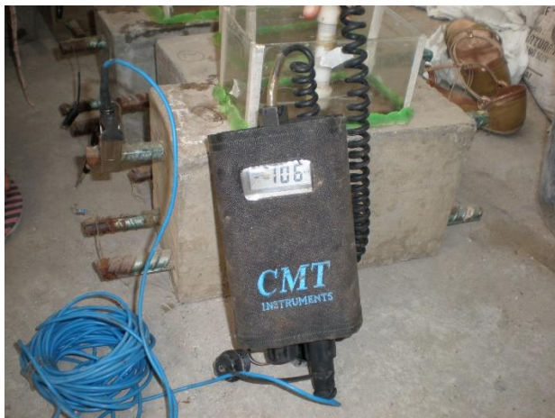
Gambar 6. Pengukuran half cell potential
